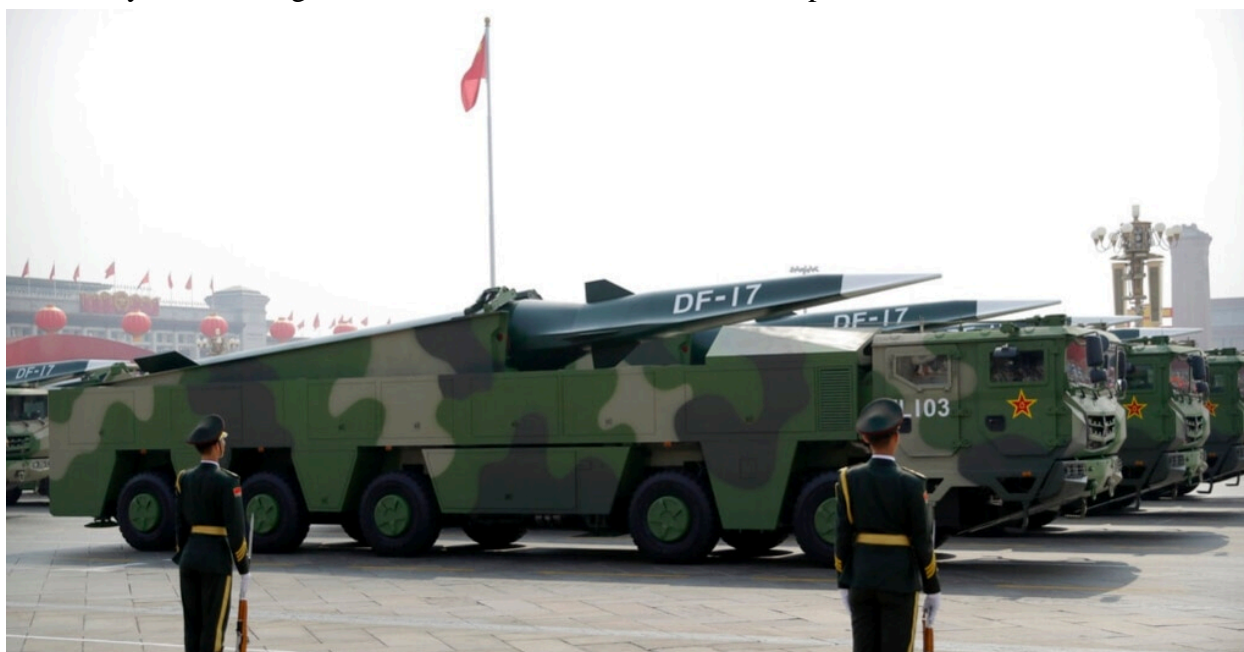
Figure 2. DF-17 ballistic missiles on military parade in 2019 mounted with hypersonic vehicles (AP).
